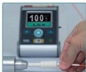
calibrate the FOX using the internal POWER METER.
